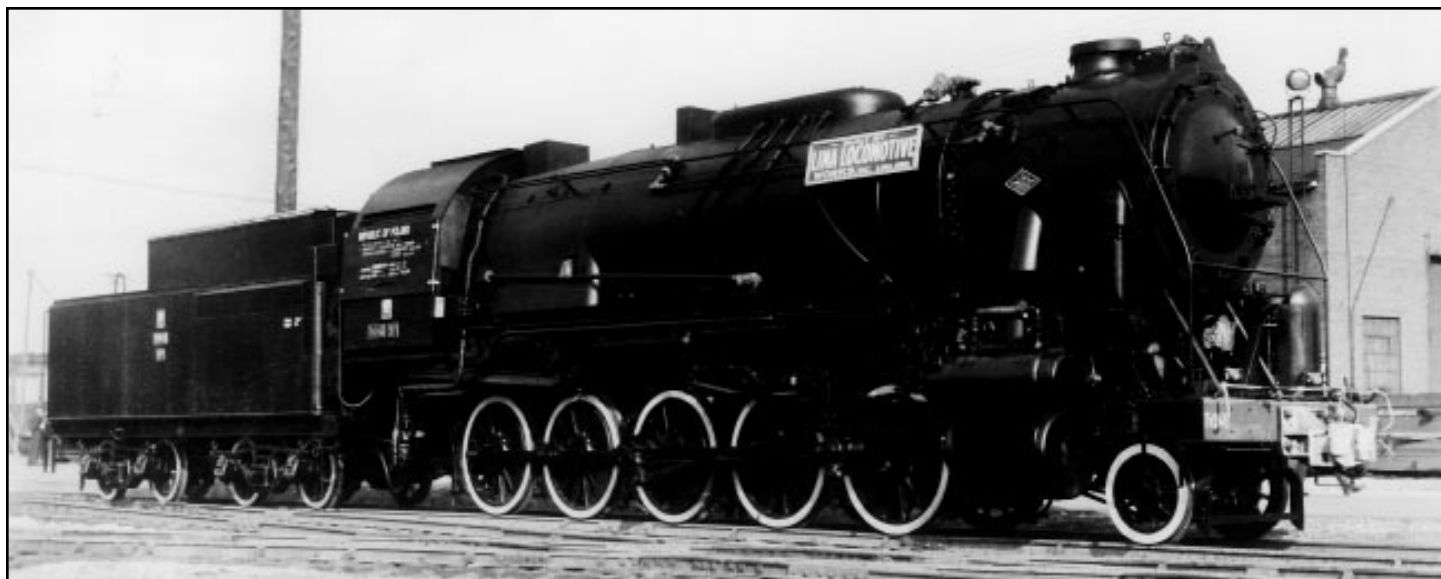
Since several of my family members are interested in transportation, some of my newsletter research involved a brief history of railroads in Poland. This particular Polish locomotive has a 2-10-0 wheel arrangement and was built in the United States by Lima Locomotive Works in October of 1947.
